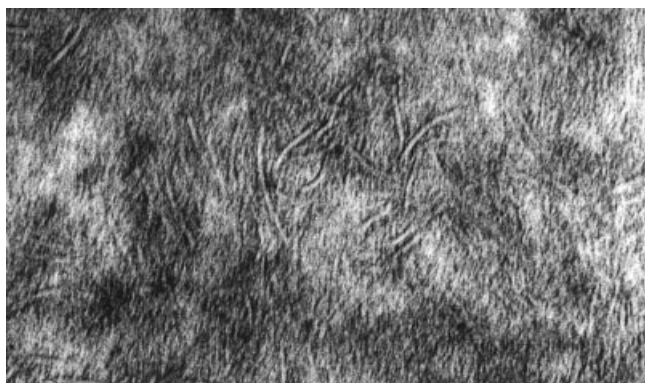
Figure 1 Morphology of the primary extruded PE tube before orientation, showing thin lamellae with no spherulitic superstructure ( \times 66,000 ).
